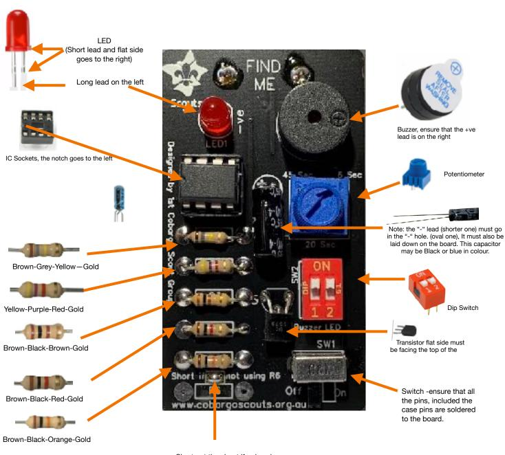
Short out the shunt if only using 2\*AA batteries - refer to the circuit diagram for more information
