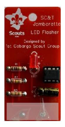
10-15mm wide tape over the battery holder pins
