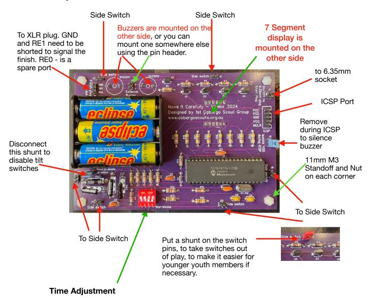
The countdown timer can be adjusted to start from 1 to 15 minutes. This is done in Binary on the Dip Switches. If you accidentally set it to 0, it will start at 1 minute.
